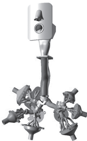
Fig. 1. Visualization of the Brno lung model – the variant of the segmented replica of airways serving for measurement of inhaled particle deposition.
