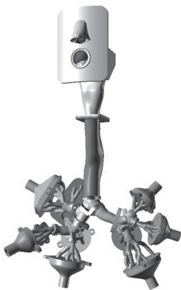
Fig. 1. Visualization of the Brno lung model – the variant of the segmented replica of airways serving for measurement of inhaled particle deposition.
